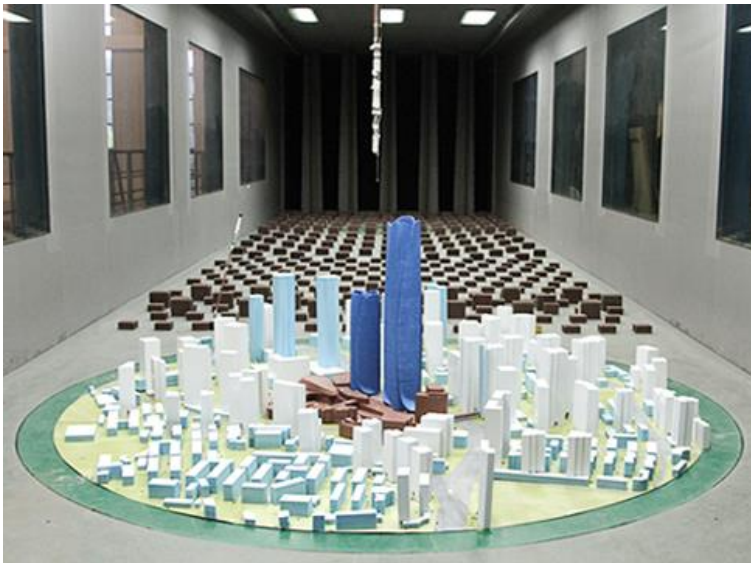
Boundary Layer Wind Tunnel test platform http://www.ccea.zju.edu.cn/cceaenglish/2016/0324/c6034a426975/page.htm
