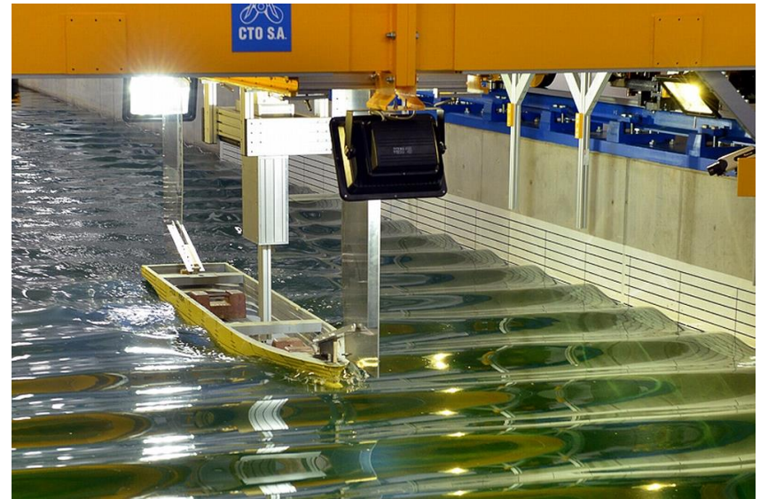
Ship model test towing tank http://www.polandatsea.com/ship-model-towing-tank-opened-at-gdansk-university-of-technology/
