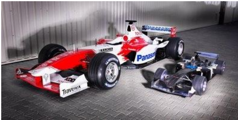
Panasonic Toyota F1 Car and 50% Scale Wind Tunnel Model.
